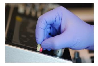
**IMPORTANT** All software and data is read from / written to the card, and the SSP needs the card to be in the slot at all times, otherwise it will stop running and can potentially crash. Pulling
