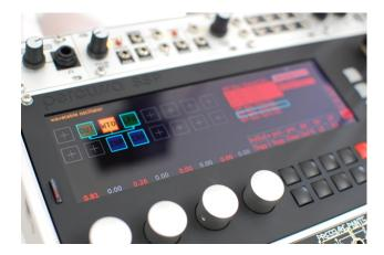
In the photo below, the selected module (WT Osc) can be modulated in X, Y, Z and Amp, and send its signal to the output module (modulation outputs, output: input).
